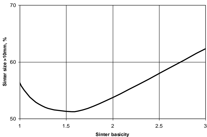
Figure 3. Relationship between sinter strength and sinter basicity. (1)
