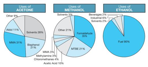
Figure 1.13. Uses of acetone, methanol, and ethanol (MMA = Methyl Methacrylate; MTBE = Methyl ter-Butyl Ether).
