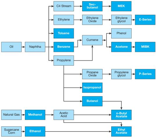
Figure 1.12. Simplified flowchart on how principal solvents are obtained.
